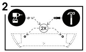
Drill the two holes with a ¼" drill bit, insert wall plugs, hammer wall plugs until flush with wall.
