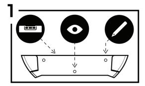
Use centre hole to find position. Keep Disc Display level, mark position of mounting holes.
